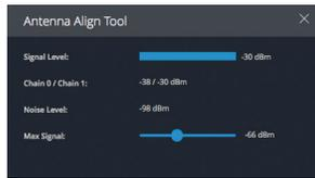
**Signal Level** Displays the signal strength of the last received packet.
