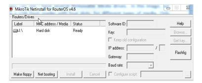
The Flashfig program can be accessed right in NetInstall as shown above.
