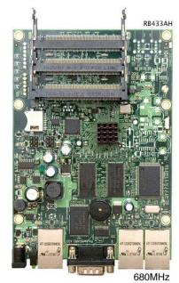
own radio card. The RouterBOARD 433, as shown to the right, includes three Ethernet and Mini-PCI Slots.
