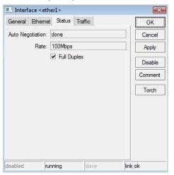
In the Ethernet status window, you will see the current status of your Ethernet port. In this example, we have performed auto-negotiation. We have a link rate of 100Mbps, and are running Full-duplex.
