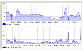
the image to the left that we have both response times in pings to this device as well as CPU usage in the top graph. Also, you can use your scroll wheel, if your mouse has one, and place the mouse cursor over the graph. By scrolling you can change from the past hour graphs to the past day, week, month and year.
