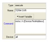
MSTSC, or terminal services. I do use Dude to monitor windows servers and having the ability to right click on the device and term serv right into the server makes it very simple. MSTSC uses a command line of *MSTC /v:address*. It is very simple to build this tool. I click the plus, to add a new tool, and then give it a name. Now I simply enter the command line, along with the address variable.
