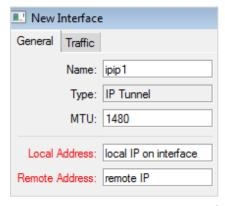
the other side of the tunnel. You will have to implement other kinds of checking, such as pinging or ARP to verify that this tunnel is running.
