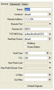
Specify the instance that you will be using, the remote IP for your peer, as well as BGP port to be used, the remote AS, and the MD5 key. Once you do this, you should be able to establish a BGP session. This is very fast and secure and you should have routes quickly.
