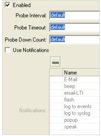
single or multiple services are down, but at least one service is up, then the device will be considered partially down. Under the Polling tab, you have options to specify how often to probe the services that you have selected on the next tab, as well as what notification options this device should use. By default, your polling options will be defaulted, this means whatever network map the device is on, it will inherit the polling settings of that map.
