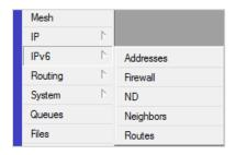
In order for your RouterOS system to support IPv6, you will have to install and/or enable the IPv6 package. In most system the package is already installed, but not enabled. By enabling the package and rebooting your router, it will enable the IPv6 feature set.
