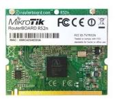
hardware. The newest Radio card is the R5N. This radio card can run in both 2.4 and the 5 gigahertz spectrum. It will run standard IEEE modes such as A, B, G, and even the prestandard of N.
