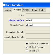
To create a virtual-AP, simply click on Interfaces → Add → Virtual AP. The main three settings you will need are the new SSID, what actual radio card you will be transmitting this new virtual SSID from, and the security profile. All of the other settings are the same as any other wireless interface. You can form WDS connections as well with a virtual AP. Once you create this interface, you will either need to place it into a bridge group, or place IPs and other Layer 3
