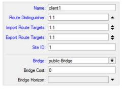
configured. We don't need to make VPLS interfaces with the BGP VPLS system, that's the point of the BGP; it will create those as necessary. The client systems would be configured the same way, however, the site ID would be different for each site.
